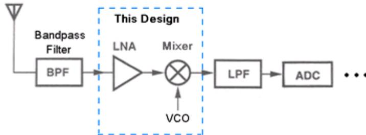
Fig. 1. a typical architecture for a RF receiver
